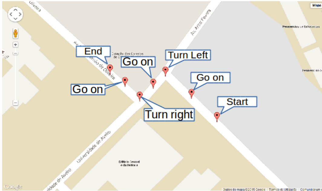
Figure 4.2: Application Example of possible solution, in which each waypoint, from the start till the end has an instruction associated
