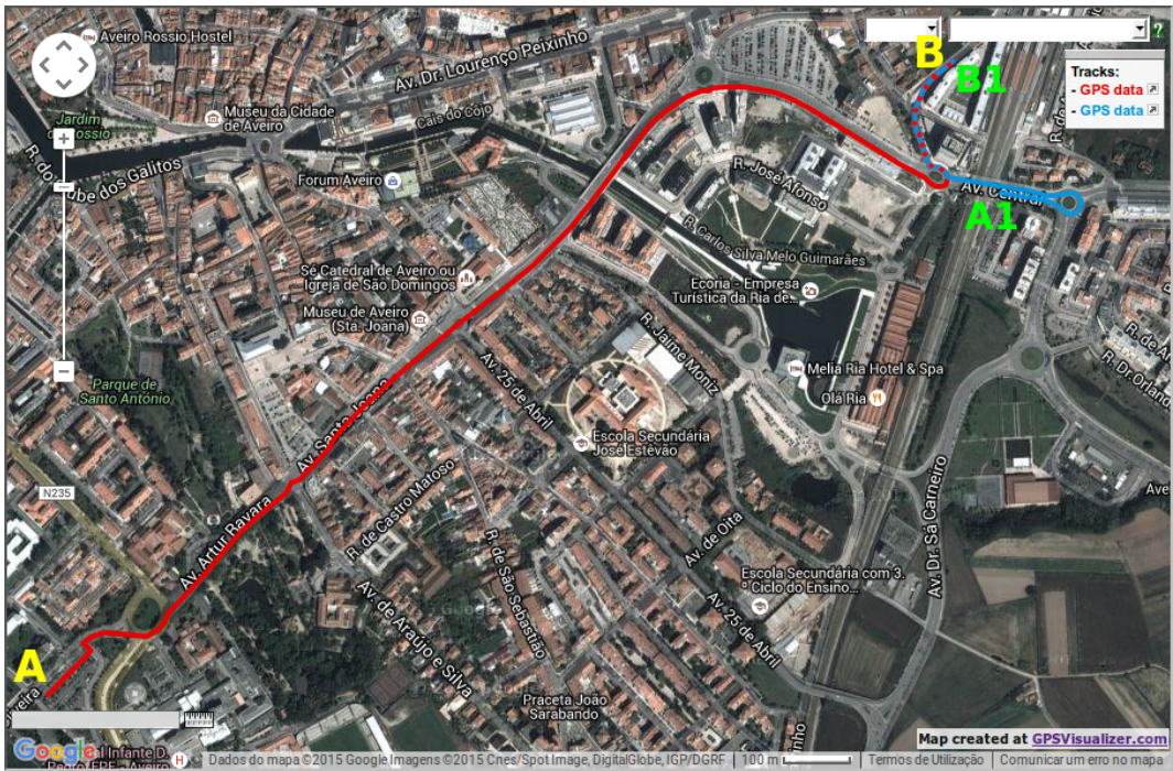
Figure 5.1: First mission to test the system. The route was from point A to B. The original route (red) was ignored at a certain point and a new route was generated (blue) from A1 to B1.
